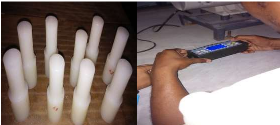
Fig 2. Machined specimens and Surface roughness test of nylon-6/6
