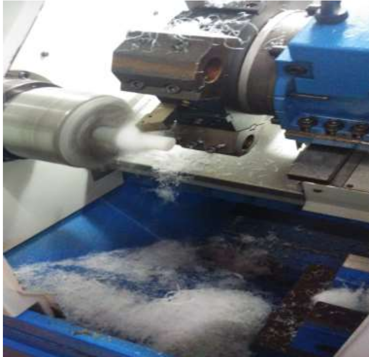
Fig 1. Turning of nylon-6/6 in CNC lathe
